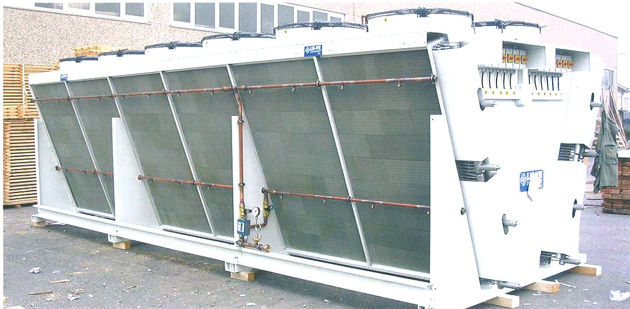
Fig.4: A large CO 2 gas cooler ready for shipping at LU-VE workshop.
